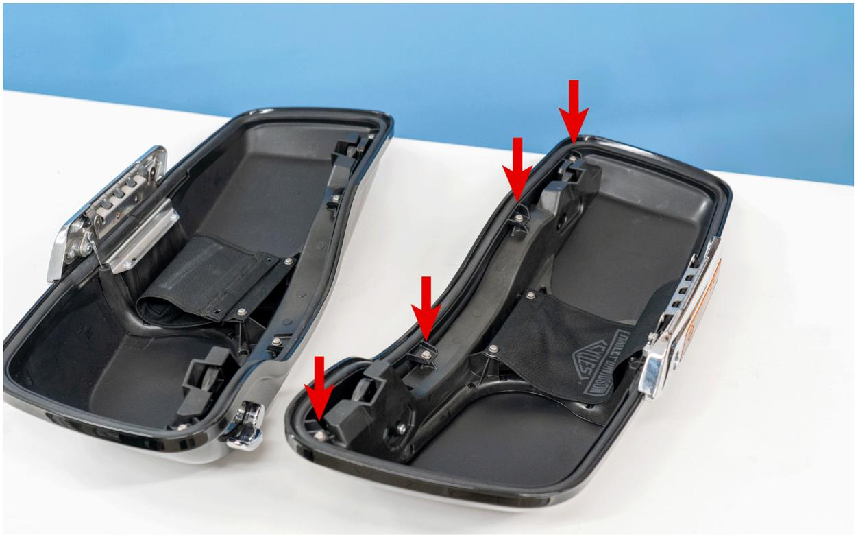
**5.3.3** Remove the two screws and carefully detach the two edges of the seal using a cutter to free the hinge.
