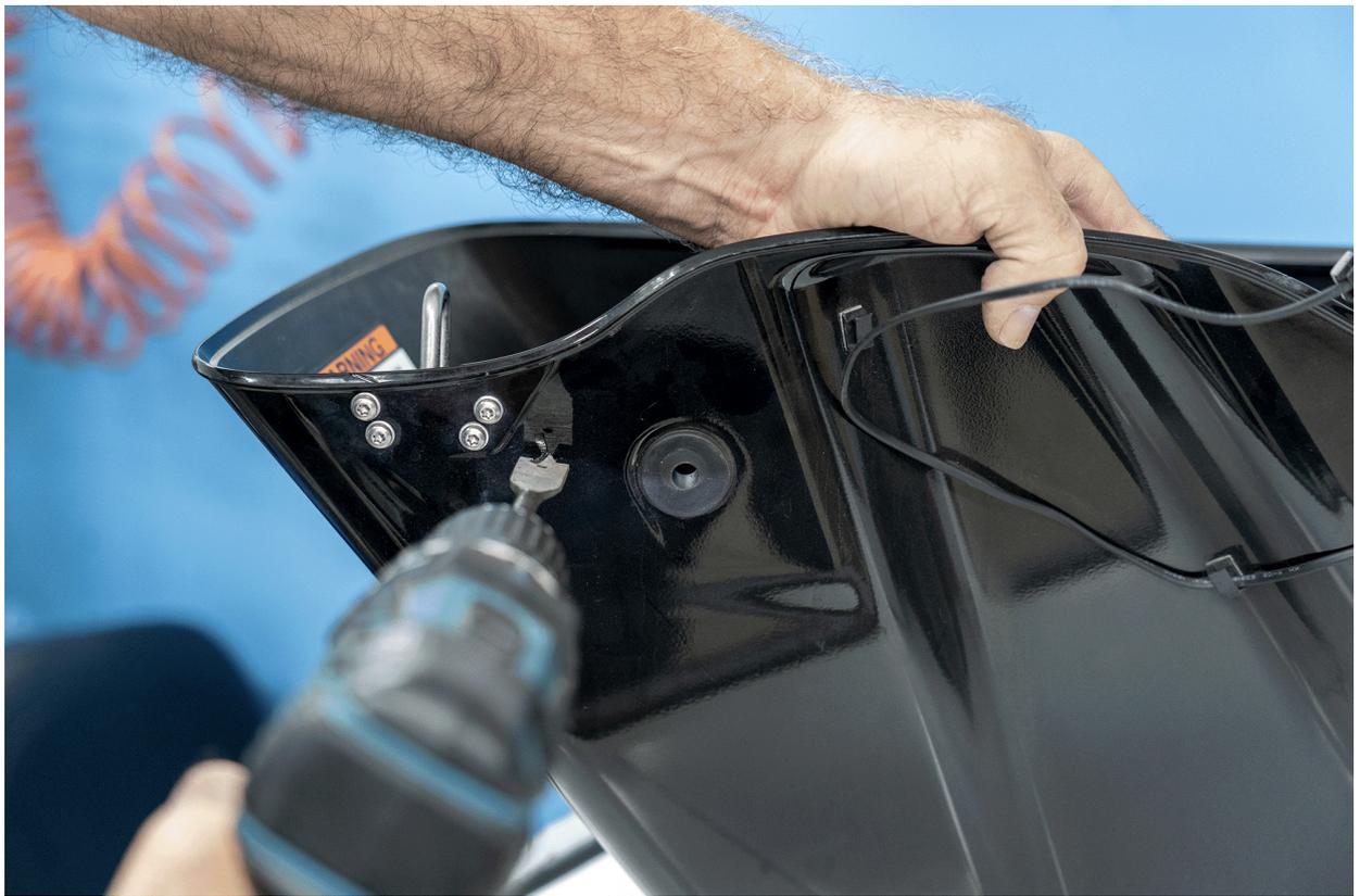
**5.11.4** Secure the grommet with a cable tie to prevent the wiring from slipping out.
