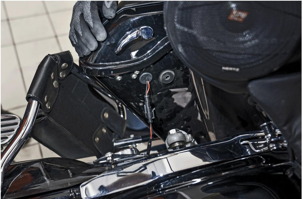
**5.13.3** Secure the Y-harness with cable ties, leaving one end unfixed for the bag, ensuring it is easily accessible but also allows for neat cable management.
