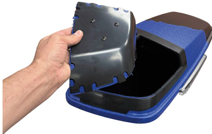
Be careful not to let the tool jump out to avoid damaging the cover. Using a variable-speed jigsaw is essential for good control.
