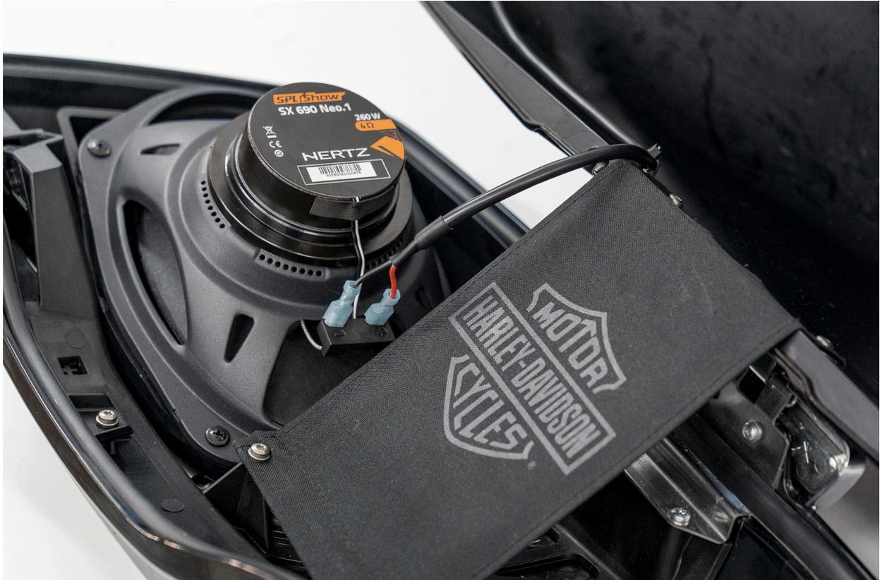
**5.12.2** Route the wiring as shown in the image below to avoid obstructing the lid's proper opening. Secure it to the front of the lid strap using adhesive cable tie mounts (not included in the kit). Use two additional cable tie mounts to secure the wiring around the front side of the bag to the exit point.
