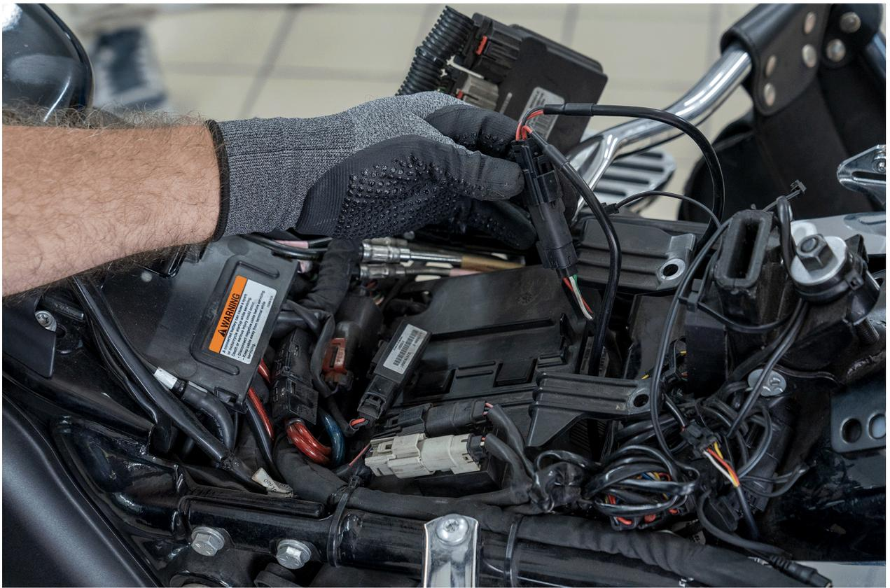
**5.13.2** Connect the Y-harness to the saddlebag. Pay attention to the wiring path on the motorcycle and where it will end up during riding. Ensure that the speaker wires do not come into contact with hot or moving parts of the motorcycle.
