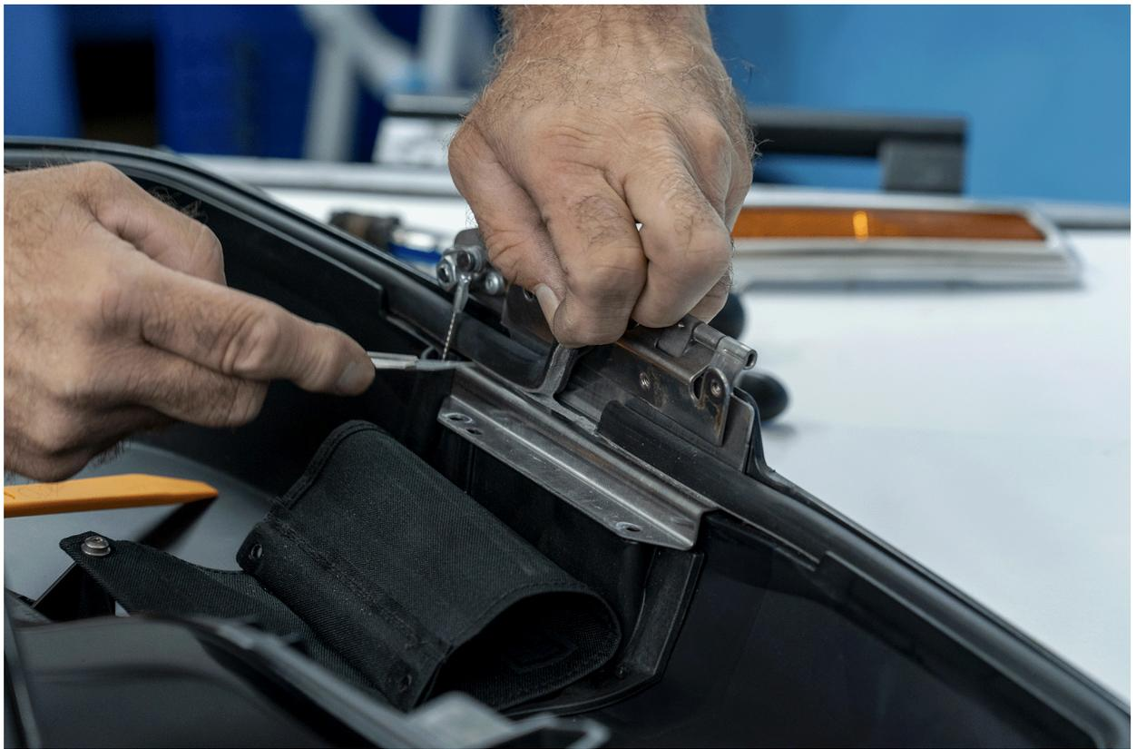
**5.3.4** At this point, the hinge can be removed.
