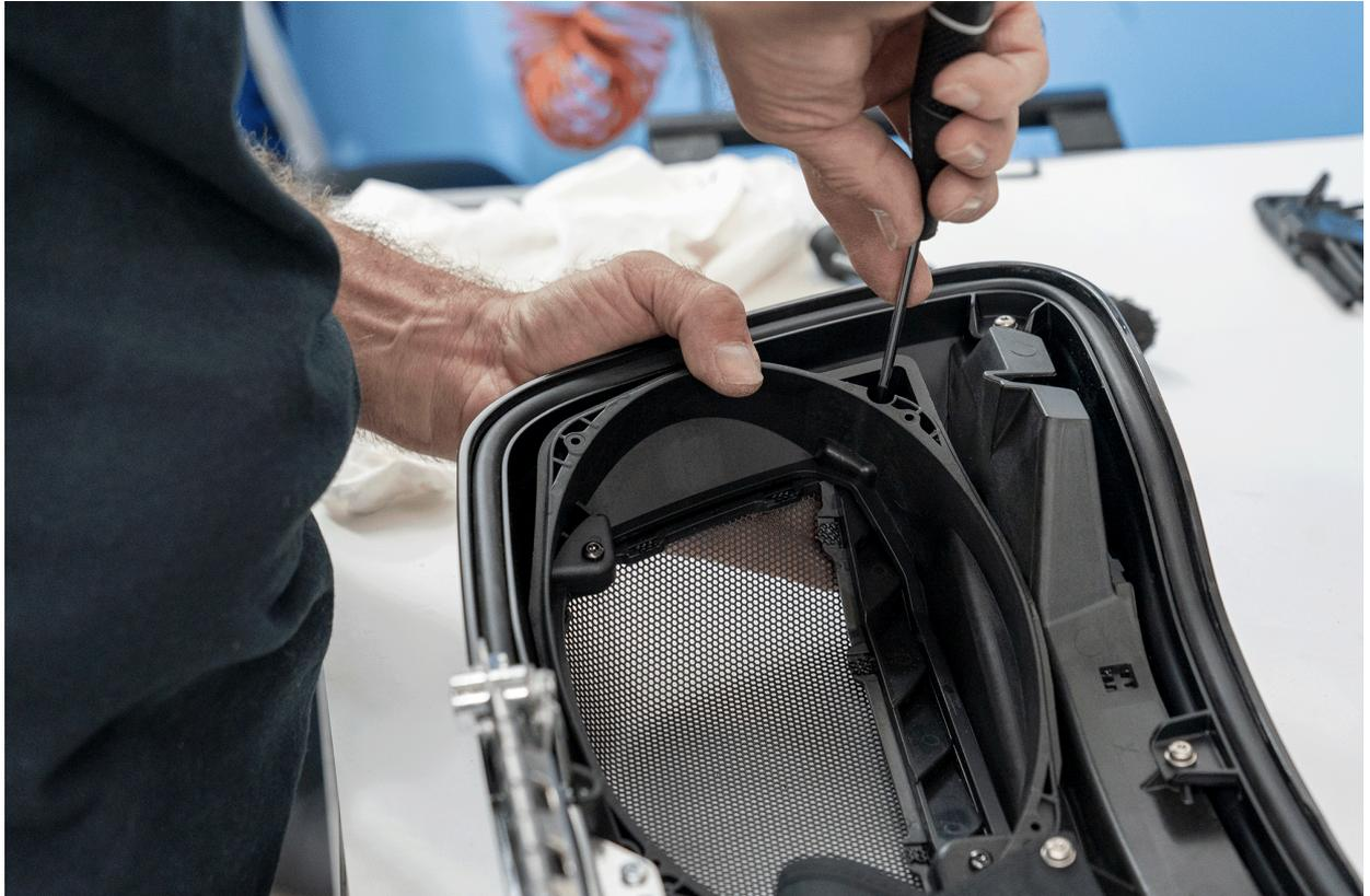
**5.8.2** Carefully attach the 6x9 adhesive gasket to the speaker mount to prevent water infiltration.
