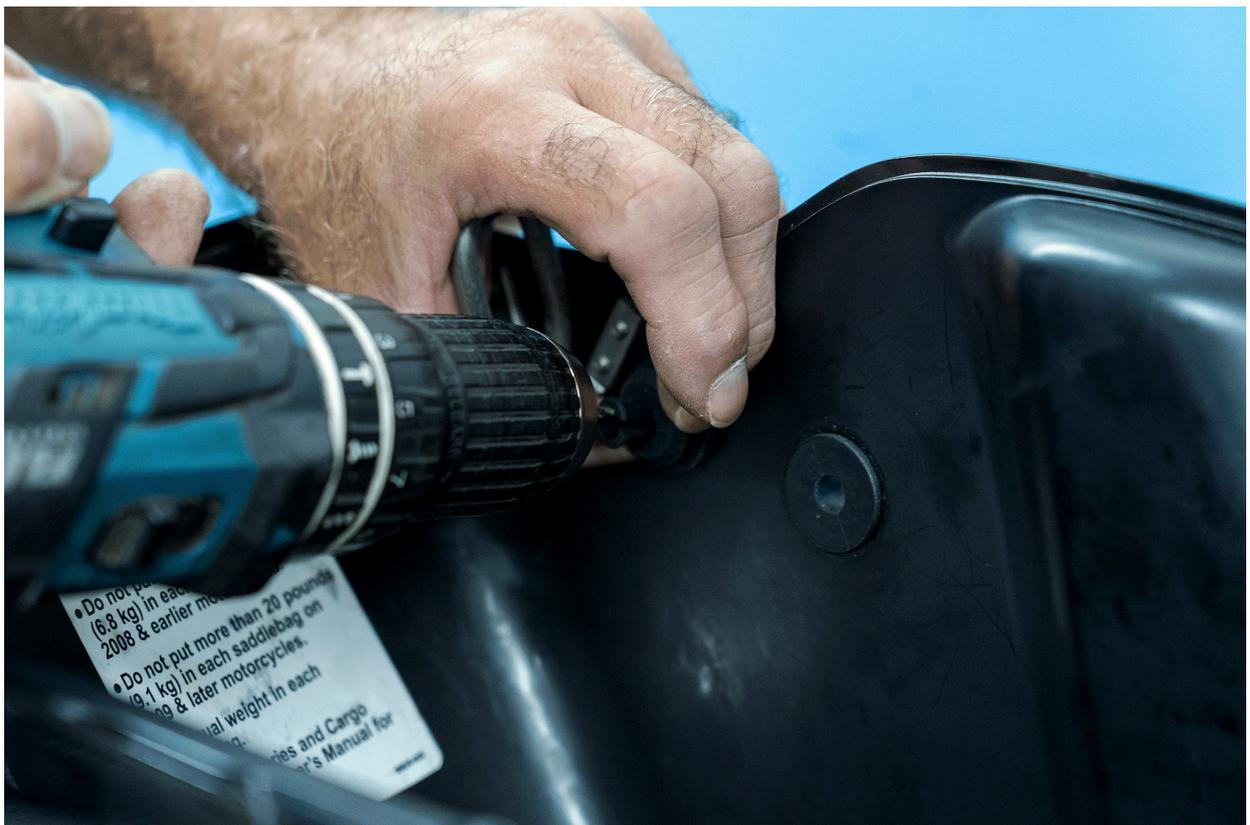
**5.11.3** Enlarge the hole with a 15/16mm drill bit, reinstall the grommet on the wiring, and pass it through the hole.
