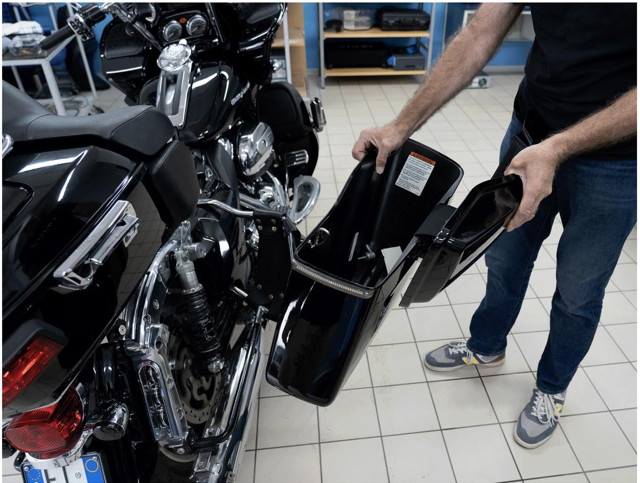
**5.1.2** To facilitate the wiring, unfasten and remove the side cover by pulling it towards you as shown in the image.
